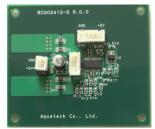
BD202412-S is driver board used to connect the motor and power supply, and to control the motor via external control signals.
