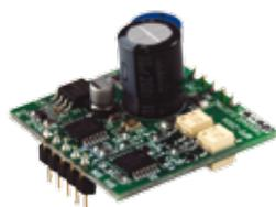
The MPD-200A is a compact driver board. It is a high voltage circuit board, specifically developed for piezoelectric micropumps. It generates the necessary output voltage of 250 Vp-p, 40 Hz to operate the pump from a 5 VDC input voltage.
